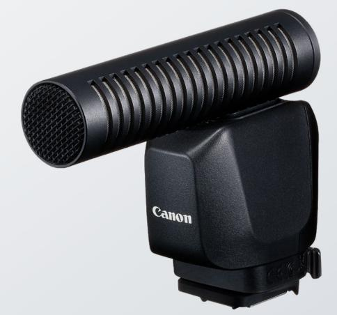
transmission of audio signal from the microphone. This allows for a battery-less and cable-less design, eliminating the risks of running out of battery or accidental detachment of cable. There are three mic directions to select from – shotgun, 90 degrees and 120 degrees. All settings are done via the camera menu and there is a dedicated Menu button at the back of the microphone to instantly trigger the mic setting page in the camera menu.
