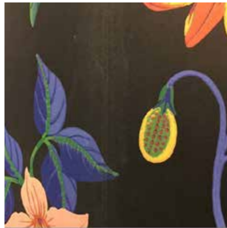
Glue residue stains
