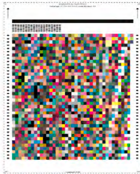
FIGURE 18: ICC swatch print with 1485 patches
