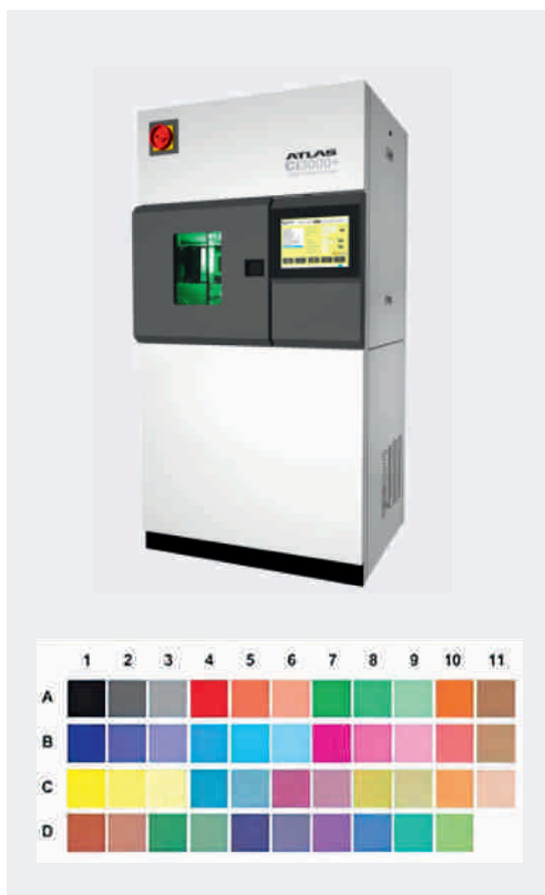
FIGURE 27: Accelerated-testing cabinet and lightfastness test chart CMYK
