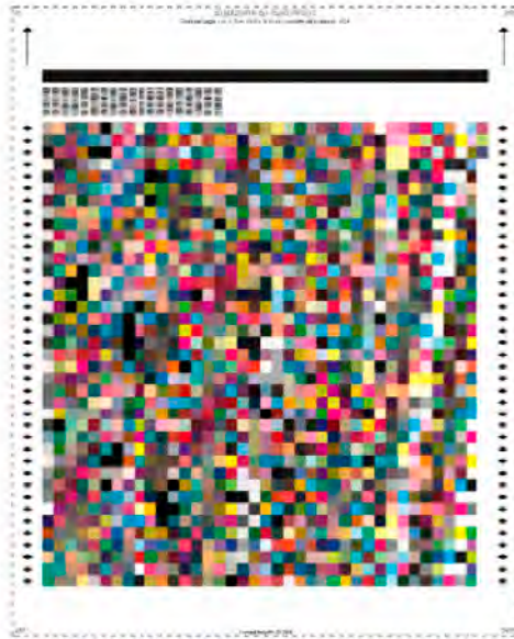
FIGURE 20: ECI2002CMYK test chart with 1485 patches
