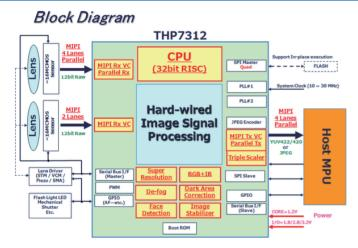
The THP7312, a high-performance image processing ISP designed by THine Electronics, is capable of high-speed image processing using a dedicated pipelined engine. A wide variety of image processing functions make it possible to maximize the performance of Canon image sensor.
